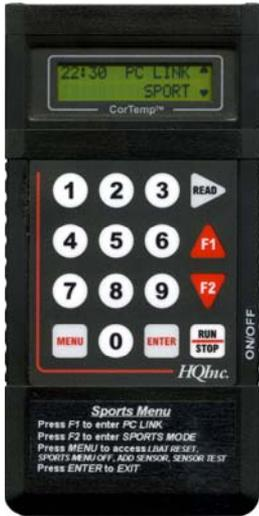
The CorTemp™ Data Recorder receives the signal from the CorTemp™ Core Body Temperature Sensor and converts the signal frequency into digital temperature data. This temperature data is displayed on the recorder LCD screen with a resolution of 0.01 degree. The recorder operates within environments between 10 and 50 degrees Celsius. User initiated sampling of temperature / heart rate is displayed for real time monitoring, while simultaneously saving to memory for future download and analysis.
